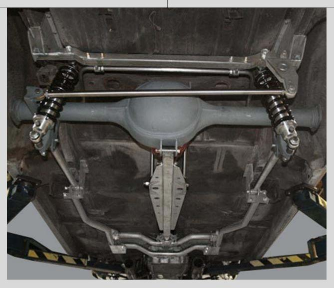
The assembly completely installed less rear axles and brakes. All parts and assemblies have been fitted and installed. Now after components have been painted or powder-coated final assembly will be much faster and no tweaking will be necessary.
